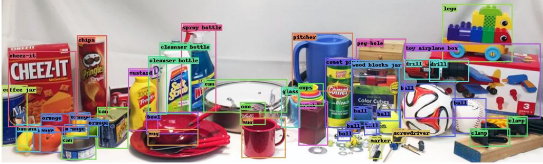
Figure 1: Demonstration of our method on YCB objects [6]. The model is trained on only the base categories of LVIS. A few example images of YCB objects are provided as novel categories during inference only.
