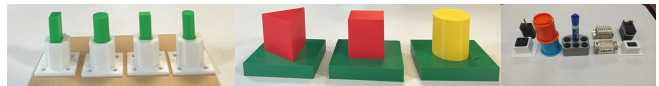
Fig. 6: (left) 3D printed objects from IndustReal [9] with 0.5 – 0.6 mm tolerance. (middle) 3D printed custom objects with 2 mm (Easy), 1 mm (Medium), and 0.1 mm (Hard) tolerance. (right) Household objects not seen during training.
