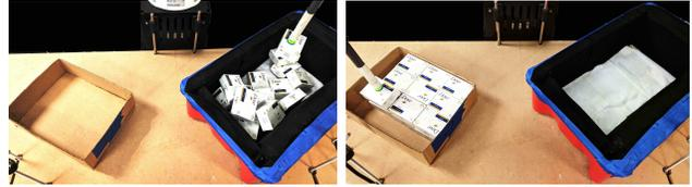
Fig. 1. The product packing problem for cuboid products: initial configuration (left), and achieved goal configuration (right).
