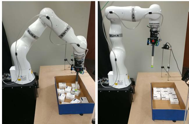
Fig. 1. The product packing problem for cuboid products: initial configuration (left), and achieved goal configuration (right). Experiments are performed using a *Kuka* robotic arm, equipped with a minimalistic end-effector and a depth-sensing camera *SR300*.
